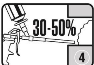
4. It should be considered that the foam would expand 30-50%. If you are filling a gap wider than 5 cm, work in layers. Apply the second layer once the first one has hardened. Once the foam has hardened, cut it with a sharp knife and finish with plastering, covering, painting, etc.
