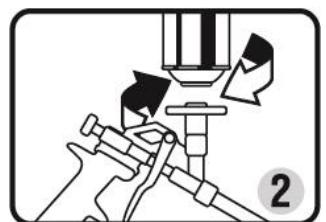
2. Press the trigger and let the foam flow through (ca. 2 seconds). This fills the foam into the extension tube. The pistol is now ready for use. During foam application hold the pistol with the can in vertical position. The output of the foam can be regulated with the trigger and controlled with the adjustment screw on the back side of the gun.
