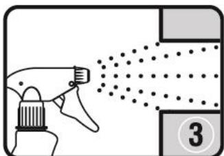
3. You can speed up the process of hardening by spraying the foam with water. When replacing the can, shake the new can vigorously, unscrew the empty can and immediately replace it with new foam can. The can replacement has to be fast to prevent that PU-foam can harden in the adapter. Hardened PU-residues in front of the nozzle can be removed only mechanically.
