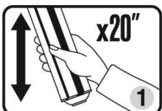
1. Surfaces should be clean, free of dust, grease and other impurities. Dry and porous surfaces should be moistened with water. The optimal temperature of can at work is 20–25°C. At lower temperature put the can into warm water (max. T=40°C) for about 20 minutes. Before use shake can thoroughly (about 20 times) with the valve upside down and screw it onto the gun.
