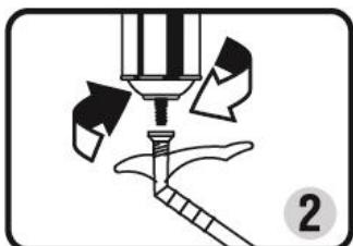
2. Press the trigger and let the foam flow through (ca. 2 seconds). This fills the foam into the extension tube. The pistol is now ready for use. During foam application hold the pistol with the can in vertical position. The output of the foam can be regulated with the trigger and controlled with the adjustment screw on the back side of the gun.
