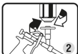
2. Remove the cap and thread the can in the gun. During foam application hold the pistol with the can in vertical position and pull the trigger to project the foam
