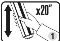
1. Surfaces should be stable, flat and clean. Before applying the polyurethane adhesive, the surface should be moistened with water. The optimal temperature of the can at work is 20-25°C. If the temperature is below that, place the can in warm water. (max. T=40°C) around 20 minutes. Before use shake can thoroughly (about 20 times) with the valve upside down and screw it onto the gun.
