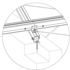
Application example 2: Direct mounting on concrete tie beams
