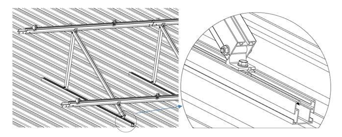
Application example 1: Assembly on PSE-C profile attached to sandwich panel roof sub-structure
