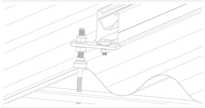
Application example 2: Mounting of the PSE-A profile on KFS-AU
