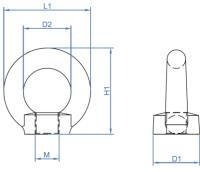
\*WLL= Working Load Limit. Is the maximum safe force that a piece of lifting equipment can exert to lift, suspend, or lower, a given mass without fear of breaking.
