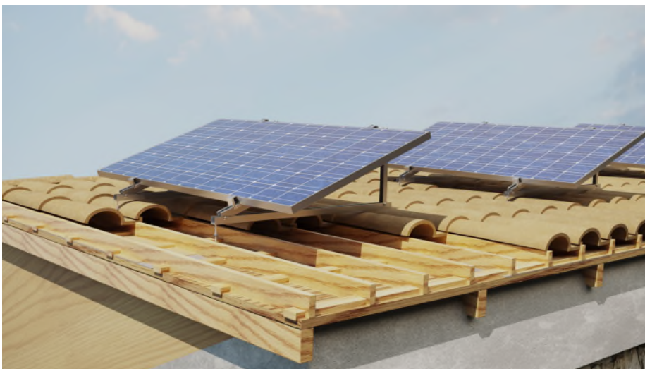
Example 2: Curved tile roof with wood substructure / Fixing with KFS-MA double threaded screw
