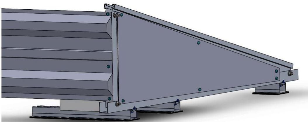
**STEP 5.- Longitudinal connection between profiles**
