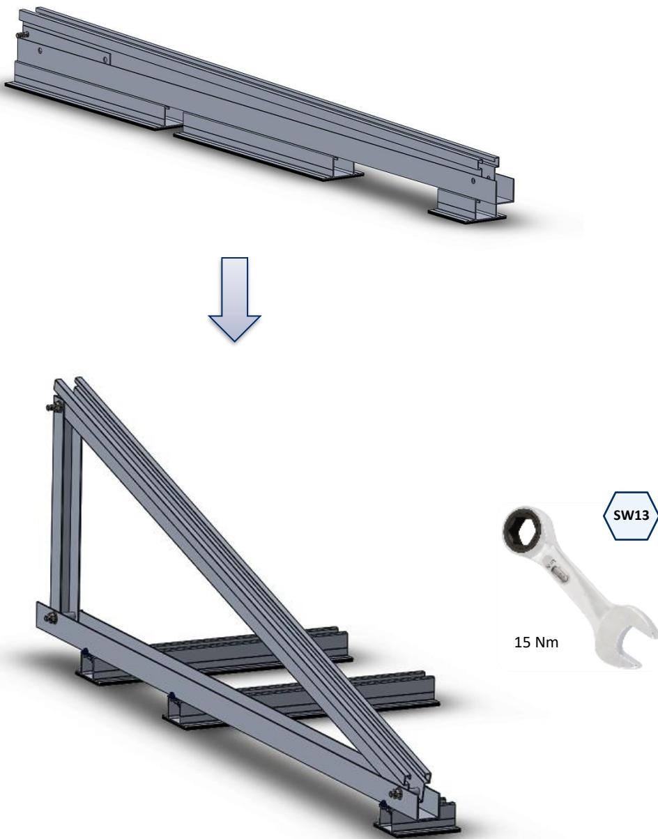
**STEP 3.- Mounting the side and rear windbreakers**
