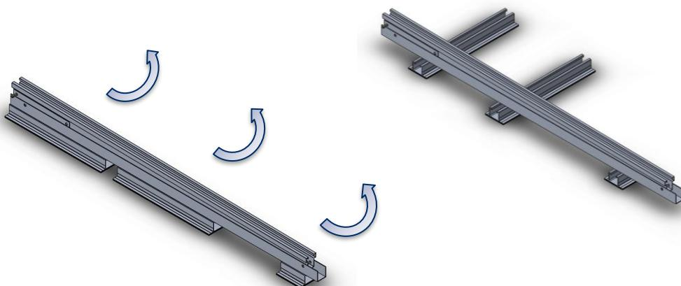
Position the support profile at 90° with respect to the lower profile, insert the stainless steel screw through both profiles placing a bushing so that when applying the tightening torque the profiles do not deform and finally place the stainless steel nut at the other end and apply a tightening torque of 15N/m.
