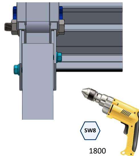
**STEP 6.- Pre-installation of staples on the profiles**
