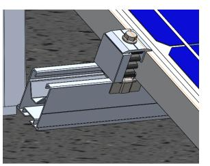
The measurement of clamps chosen should be equal to the frame height of the solar panels being installed.
