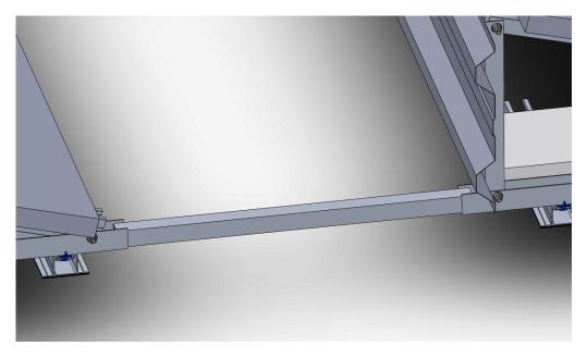
Fix the joining profile to the lower profiles by installing 2 stainless steel self-drilling screws on each side. The screws must be installed on the sides of the profile, in the shape of a cross so that they do not collide with each other. For the installation of the screws, an electric screwdriver equipped with a SW-8 hexagonal socket is needed, an installation speed of 1800 rpm is recommended.
