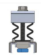
1. Place the clamp in the profile with the lower nut parallel to the profile.
