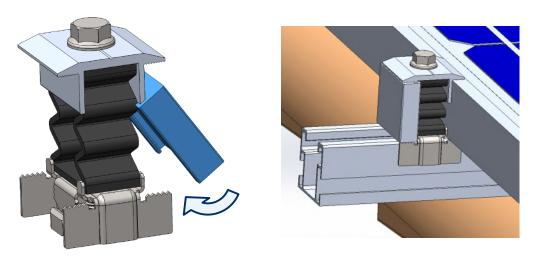
The chosen gauge size must be equal to the frame height of the solar panels to be installed.
