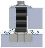
**3.** Insert the corresponding elements, two panels in the case of an intermediate clamp, or a panel and a gauge in the case of a lateral clamp.
