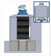
**4.** To fix the inserted elements it is necessary to turn the screw until they meet the profile. Check that the lower nut remains perpendicular to the profile.
