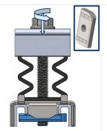
2. To fix the clamp to the profile, the lower nut must be turned perpendicular to the profile by means of the screw, the screw head is pressed down and turned. The nut has a serrated rail to secure the fixing.
