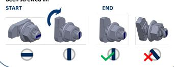
**E.** To adjust the position of the PSE-C profile, the KFS-FI connectors can be loosened. By keeping the square neck of the connector locked on the edge of the profile groove, we prevent the head from turning inside the groove when loosening the connector nut.
