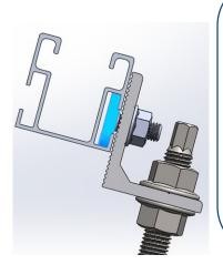
To ensure that the head of the KFS-FI connector is oriented perpendicular to the profile, there is a mark at the base of the screw. This mark indicates the final position of the head, so it must be perpendicular to the profile at the end of the installation. The mark must never be parallel to the profile or inclined once it has been screwed in.
