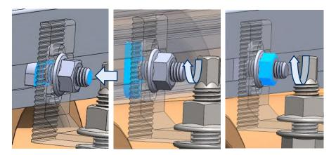
**D.** Check that the head of the KFS-FI connector is oriented perpendicular to the groove of the PSE-C profile and the square neck of the connector is correctly fitted into the edge of the groove.
