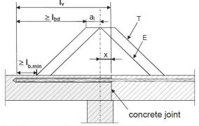
Installed condition and examples of use for rebars
