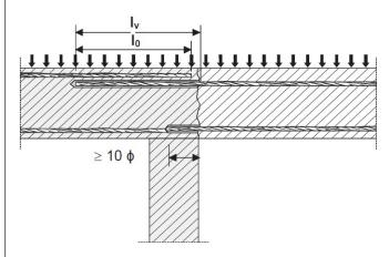
**Figure A3:** End anchoring of slabs or beams, designed as simply supported
