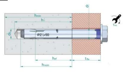
$\begin{array}{ll} d_0 \colon & \text{Nominal diameter of drill bit} \\ d_f \colon & \text{Fixture clearance hole diameter} \\ h_{ef} \colon & \text{Effective anchorage depth} \end{array}$
