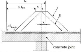
(only post-installed rebar is plotted)
