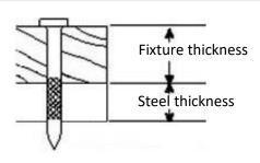
Nail length = Fixture thickness + Steel thickness
