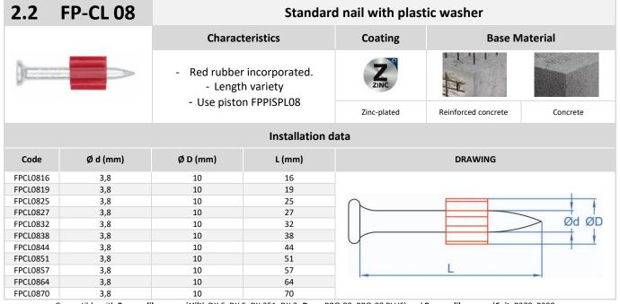
Compatible with 8mm caliber guns (*Hilti*: DX 6, DX 5, DX 351, DX 2; *Desa*: PRO-08, PRO-08 PLUS) and 9mm caliber guns (*Spit*: P370, P390, P60; *Desa*: PRO-09).
