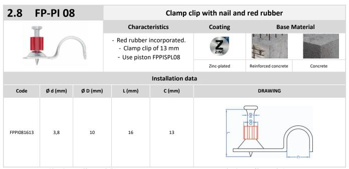
Compatible with 8mm caliber guns (*Hilti*: DX 6, DX 5, DX 351, DX 2; <u>Desa</u>: PRO-08, PRO-08 PLUS) and 9mm caliber guns (<u>Spit</u>: P370, P390, P60; <u>Desa</u> PRO-09).
