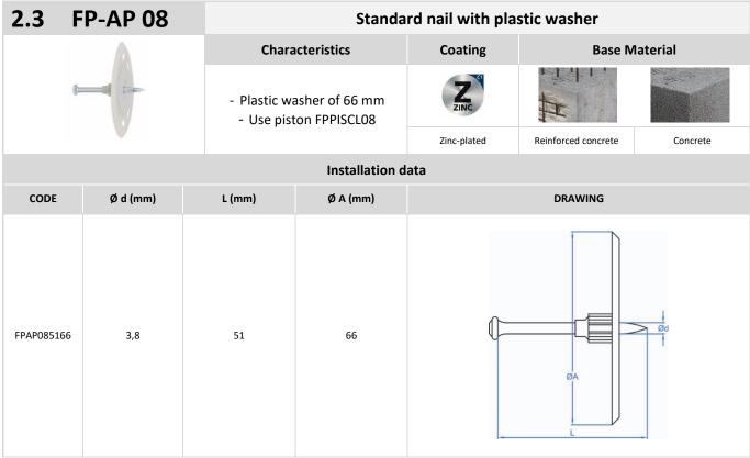
Compatible with **8mm caliber guns** (<u>Hilti:</u> DX 6, DX 5, DX 351, DX 2; <u>Desa:</u> PRO-08, PRO-08 PLUS)
