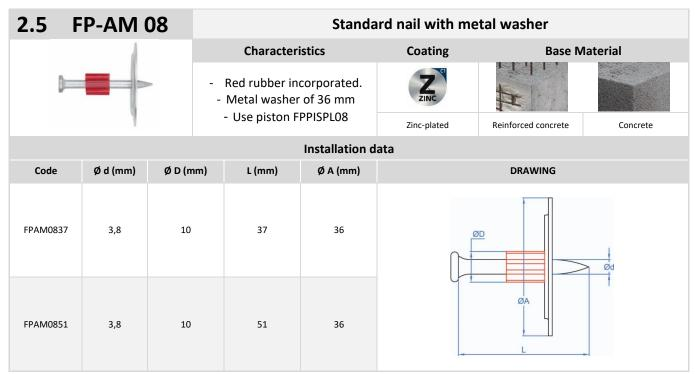
Compatible with 8mm caliber guns (<u>Hilti:</u> DX 6, DX 5, DX 351, DX 2; <u>Desa:</u> PRO-08, PRO-08 PLUS) and 9mm caliber nailers (<u>Spit:</u> P370, P390, P60; <u>Desa</u> PRO-09).
