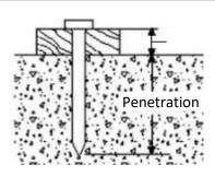
Total nail length = Fixture thickness + Penetration
