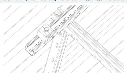
Application example 4: mounting on INDEXTRUT solar triangle.
