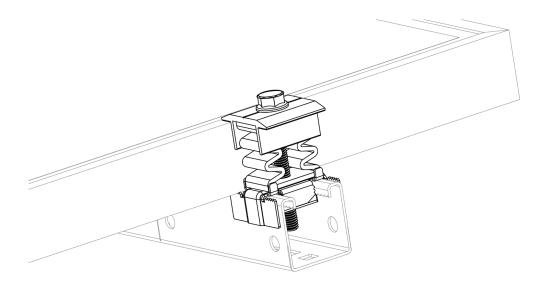
Application example 1: Mounting on a GP-XS INDEXTRUT solar perforated guide in an intermediate position.
