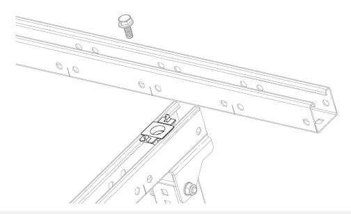
Application example 1: Mounting on a GP-XS INDEXTRUT solar perforated guide on a TRPXS412515 triangle.
