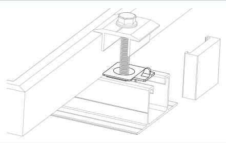
Application example 1: Mounting of a PGSA26 simple clamp at the end of the line on a PSA-A profile.
