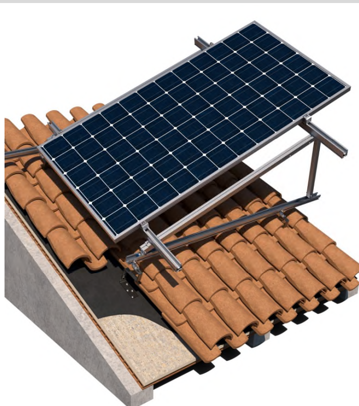
Example 2: Curved tile roof with wooden substructure / fixing with double threaded bolt KFS-MA
