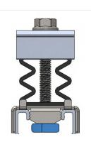
1. Place the clamp in the guide with the lower nut parallel to the guide.
