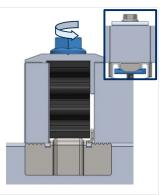
**4.** To fix the inserted elements it is necessary to turn the screw until they meet the guide. Check that the lower nut remains perpendicular to the guide.
