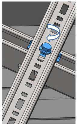
STEP 6.- Longitudinal connection between guides
