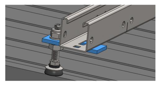
G. Fasten the GP-XS guide onto the PMO plate using DIN 603 screws (M8x20) and DIN 6923 M8 nuts.
