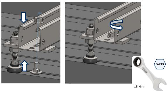
Tighten to a maximum torque of 15 Nm using a SW-13 hexagon spanner.
