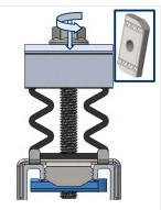
2. To fix the clamp to the guide, the lower nut must be turned perpendicular to the guide by means of the screw, the screw head is pressed down and turned. The nut has a serrated rail to secure the fixing.
