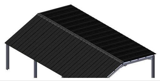
STEP 3.- Installation of the GP-XS rails and fixings
