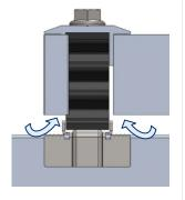
**3.** Insert the corresponding elements, two panels in the case of an intermediate clamp, or a panel and a gauge in the case of an end clamp.
