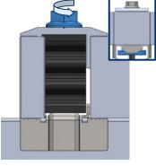
**4.** To fix the inserted elements it is necessary to turn the crew until they meet the profile. Check that the lower nut remains perpendicular to the profile.
