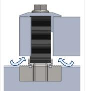
**3.** Insert the corresponding elements, two panels in the case of an intermediate clamp, or a panel and gauge in the case of lateral clamp.
