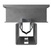
**1**. Press the panel (with the clamp already fixed) on the profile where you want to anchor it until you hear a click for each of the clamps on the module.
