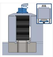
**4.** To fix the inserted elements it is necessary to turn the screw until they meet the guide. Check that the lower nut remains perpendicular to the guide.
