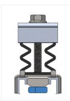
**1.** Place the clamp in the guide with the lower nut parallel to the guide.
