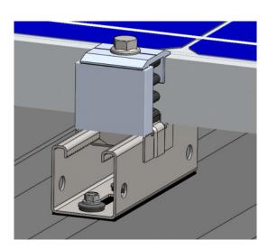
The chosen gauge size must be equal to the frame height of the solar panels to be installed.
