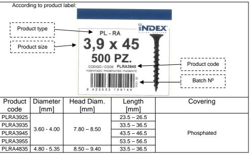
3. Intended use: To fix gypsum plasterboard, gypsum boards with fibrous reinforcement, products
